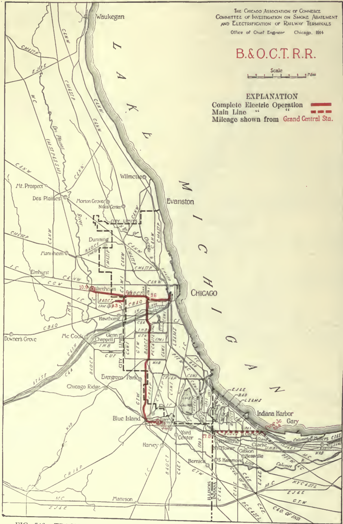
FIG. 546. TRACKAGE TO BE ELECTRIFIED BY THE BALTIMORE & OHIO CHICAGO TERMINAL RAILROAD
